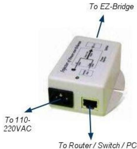
6. Connect a CAT5 cable from your computer, switch or Unitec router to the LAN connector on the wall plug POE inserter. Connect the CAT5 from the antenna to the POE connector on the wall plug POE inserter. Plug the wall plug POE inserter into a surge protected AC power source to power up the bridge
