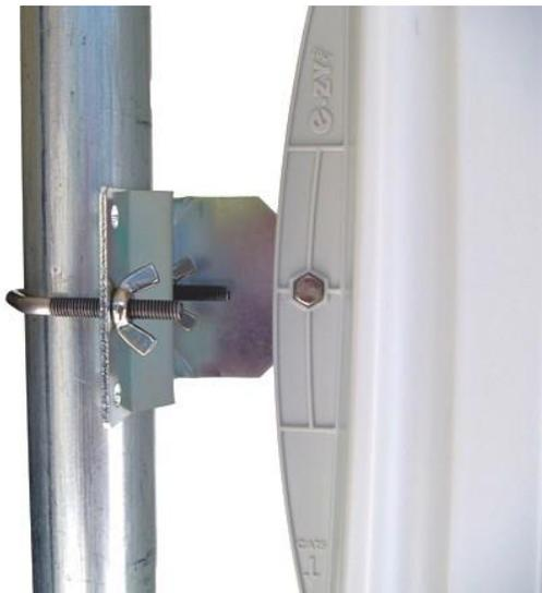
2. Mount the antenna housing to the bracket. Put the hex head bolt thru the housing back fin. Put the star lock washer so it is between plastic housing and metal bracket. Install
