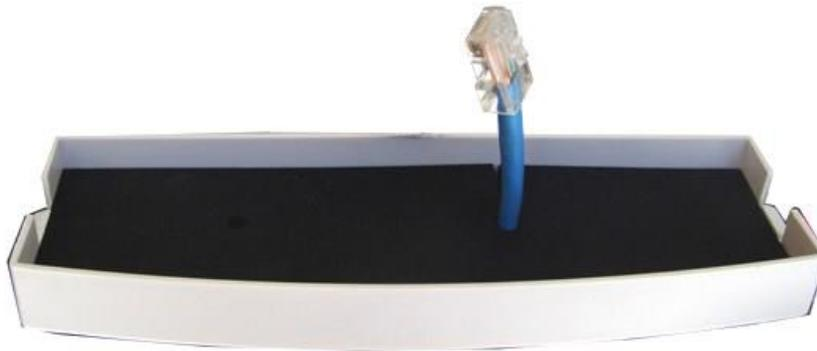
4. Route a CAT5 cable through the bottom cover and plug into the RJ45 Jack inside the unit. Keep the black gasket material in the bottom of the cover to help keep out dust and insects.
